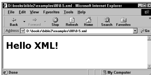
Figure 8-2: Hello XML with a DTD and style sheet displayed in Internet Explorer 5.5
