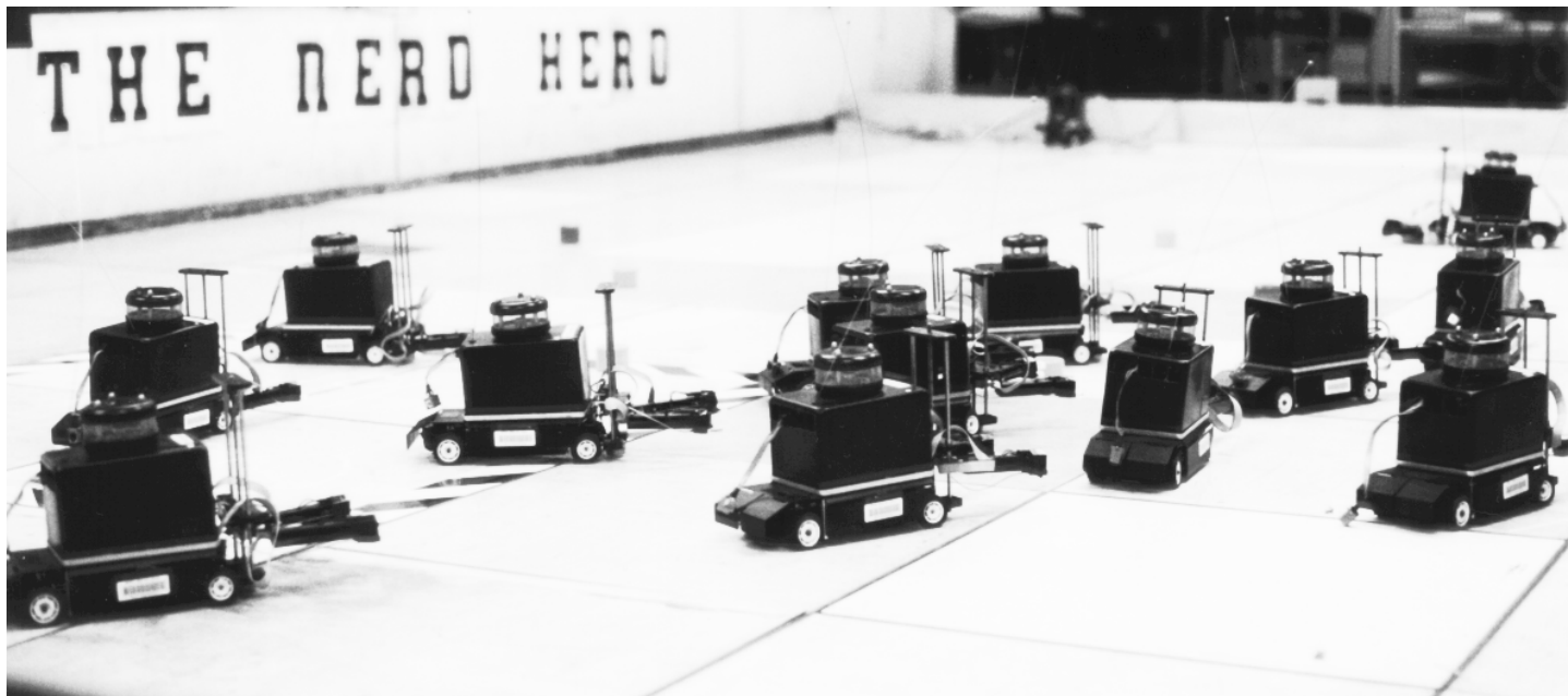
Figure 1: A group of 13 flocking mobile robots. These robots also demonstrated wandering, following, aggregation, dispersion, chain-formation, and foraging.
