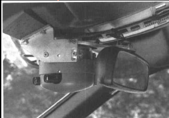
Figure 7.21 (continued) High-speed road-following autonomous robots: (A) VaMoRS, (B) vaMP, and (C) vaMP vision system. (Photographs courtesy of Ernst Dickmanns.)
