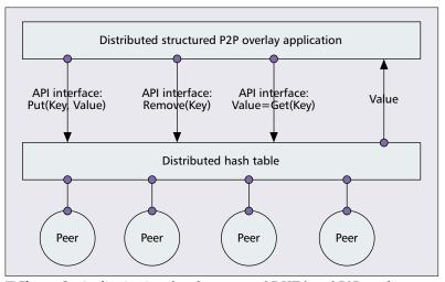
■ Figure 2. Application interface for structured DHT-based P2P overlay systems.
