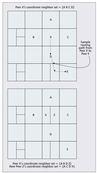
■ Figure 3. Example of 2-d space CAN before and after Peer Z joins.
