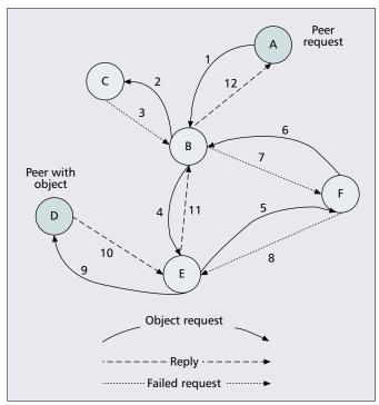
■ Figure 7. A typical request sequence in Freenet.
