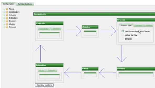
Fig. 6. The GUI of the autonomic computing self-configuration solution for virtual servers.
