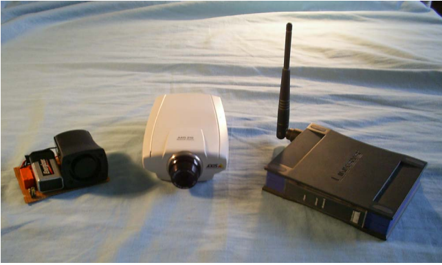
Fig. 4. Camera, bridge and alarm bell.
