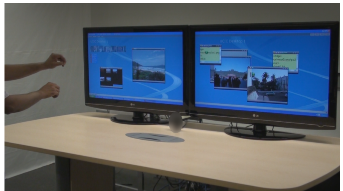
Fig. 9. Controlling Two Cursors to Move Two Windows at the Same Time.
