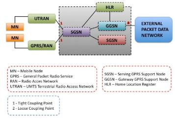
Figure 1. Coupling Architectures
