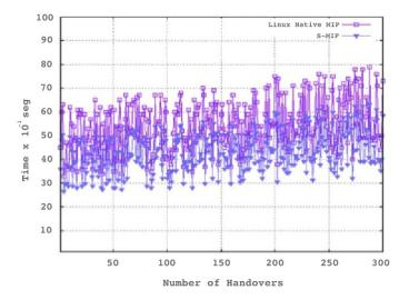
Figure 4. Delay I-MIP x Delay Linux Native MIP
