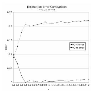
Fig. 10. Comparison of estimation errors with R = 0.25 and m = 40.
