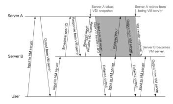
Fig. 1. Protocol timeline for a mobile station moving from Server A to Server B.
