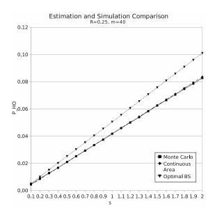
Fig. 9. Comparison of estimated and simulated  $P_{HO}$  with R = 0.25 and m = 40.
