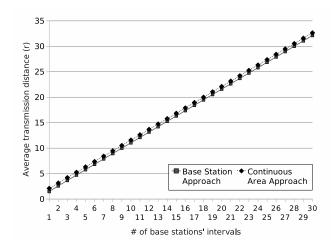
Fig. 8. Comparison of average transmission distances of different approaches covering approximately equal service area.
