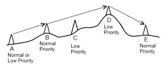
Figure 5. In this example, B is selected by the algorithm because of its priority, despite the direct communication with D.
