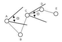
Figure 1. With a directional antenna with an opening angle  $\theta$ , vertex C aligned with E covers D, however A aligned with C does not cover B.
