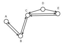
Figure 2. An example of an aligment graph. In this case, the pairs of antennas connecting A-B, B-C e C-E are aligned.
