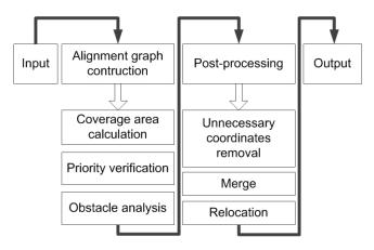
Figure 3. Flow chart of the LMP algorithm.
