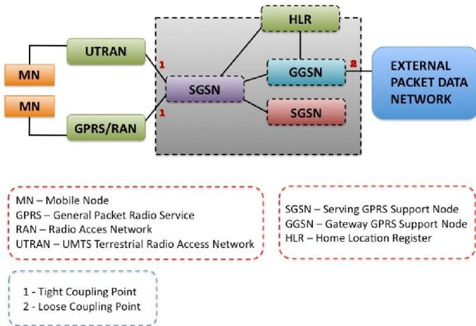
Figure 1. Coupling Architectures
