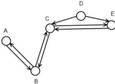
Figure 2. An example of an alignment graph. In this case, the pairs of antennas connecting A-B, B-C e C-E are aligned.
