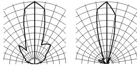
Figure 11. The horizontal (left) and vertical (right) irradiation pattern.
