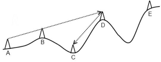
Figure 8. This example shows how D can be selected A's best neighbor, even with A not establishing a direct communication with C.
