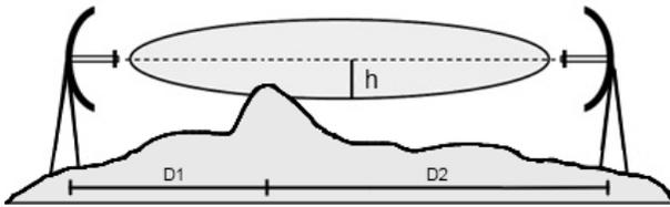
Figure 4. In the Fresnel zone, the radius  $h$  of the ellipsoid is related to the transmission frequency and distance.
