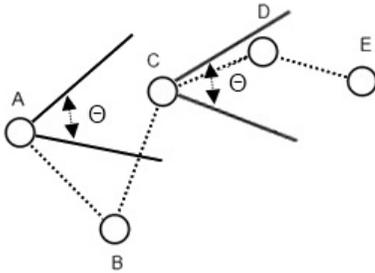
Figure 1. With a directional antenna with an opening angle  $\theta$ , vertex C aligned with E covers D, however A aligned with C does not cover B.
