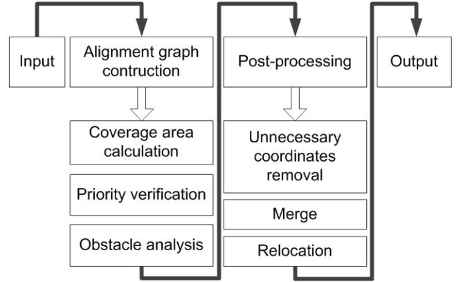
Figure 3. Flow chart of the LMP algorithm.
