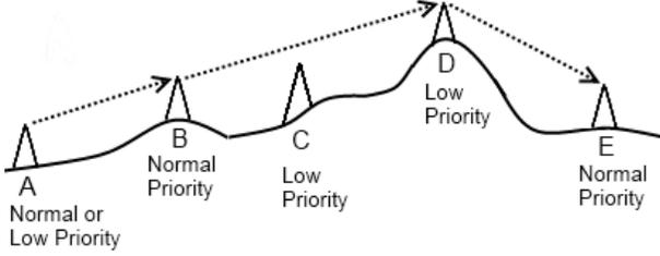
Figure 5. In this example, B is selected by the algorithm because of its priority, despite the direct communication with D.
