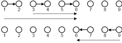
Figure 12. The communication between 5 and 6 receives interference from the pairs 1, 2 and 3, 4. When the communication occurs between 6 and 7, the interference comes from the pair 8, 9.
