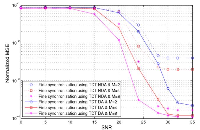
Figure 5. Normalized MSE of our fine synchronization approach in both NDA and DA modes
