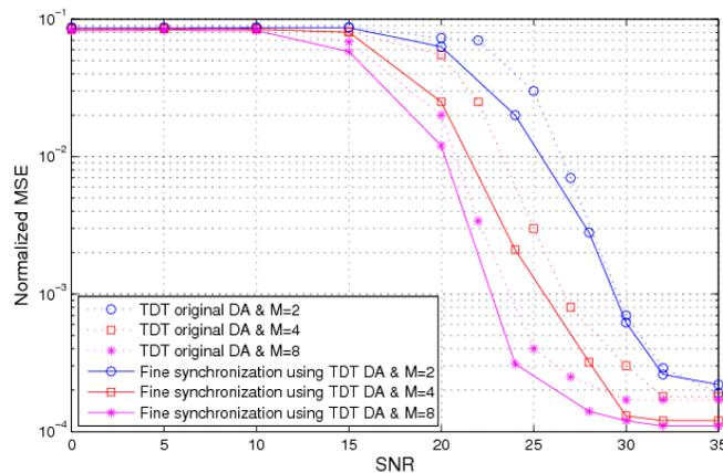
Figure 7. Performances comparison between original TDT and our fine synchronization approaches in DA mode
