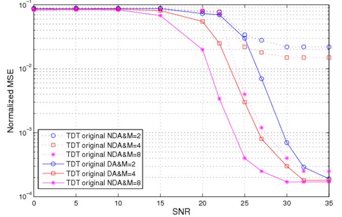
Figure 4. Normalized MSE of the original TDT synchronizer in both NDA and DA modes
