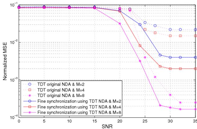
Figure 6. Performances comparison between original TDT and our fine synchronization approaches in NDA mode
