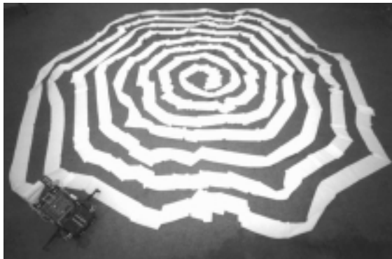
Figure 4. A spiral 'foraging' trail generated by the robot trace-maker.
