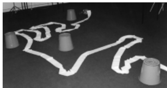
Figure 11. A robot trail generated by a combination of meandering and obstacle-avoidance behaviors.
