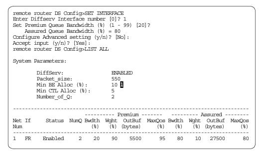
Figure 30. Enabling DiffServ on an interface
