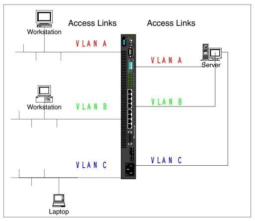
Figure 60. Port-based VLANs inside a switch
