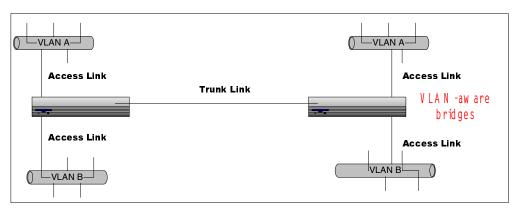
Figure 56. Port-based VLANs and trunk links
